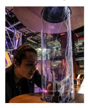
The 'lightning strike' exhibit involves electricity in a tube with a model statue inside. The tube is filled with a mixture of gases, which makes the electricity visible when there's a high voltage. I can touch the tube to change the lightning's direction, and I might feel a small shock or tingling sensation.
