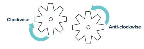
1. (b) Add a third gear, and watch the direction that it rotates. If there were 75 gears in a line, with the first gear rotating anti-clockwise, in which direction would the last gear rotate?
